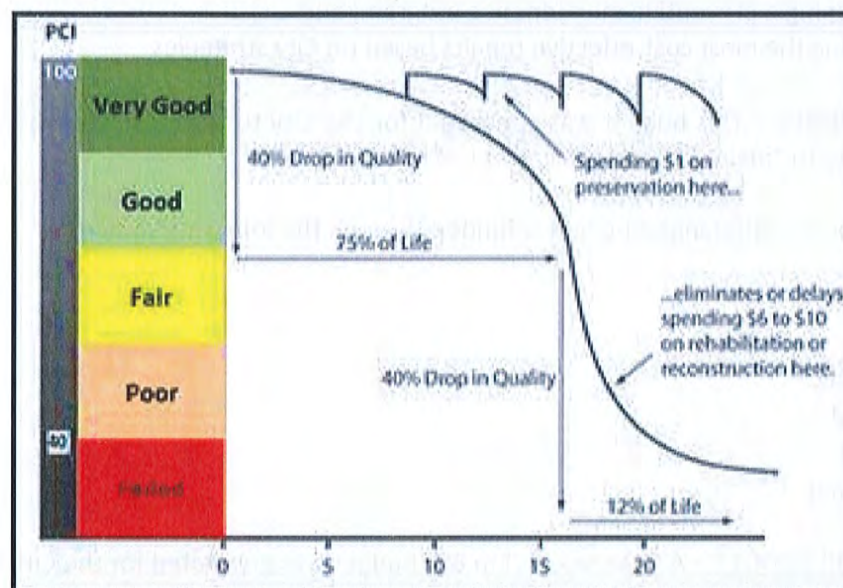
Figure 3 – Sample Pavement Life Cycle / Deterioration Rate
